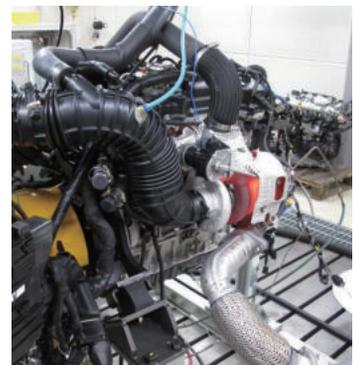
Engine Dynamometer Test
